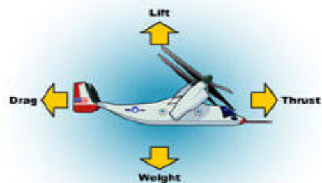
Fig: Four Forces on an Airplane (Ref: NASA)
